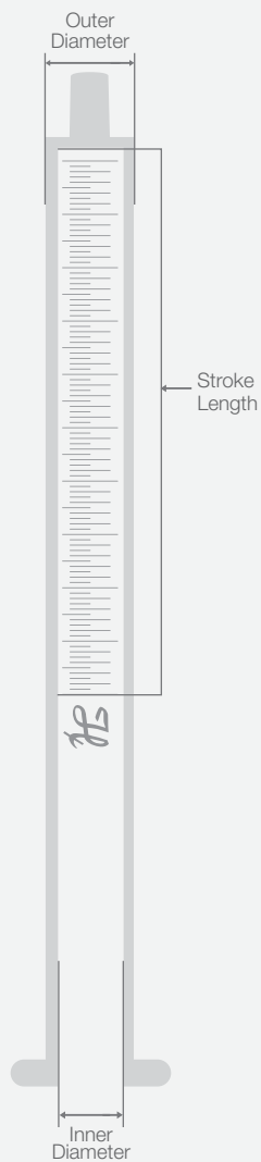
Syringes Figure 7. Syringe dimensions
